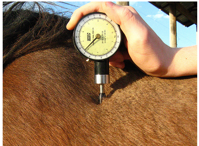
Figure 1. Application of a pressure algometer over the cranial thoracic region to objectively assess mechanical nociceptive thresholds within soft tissue or bony landmarks.
